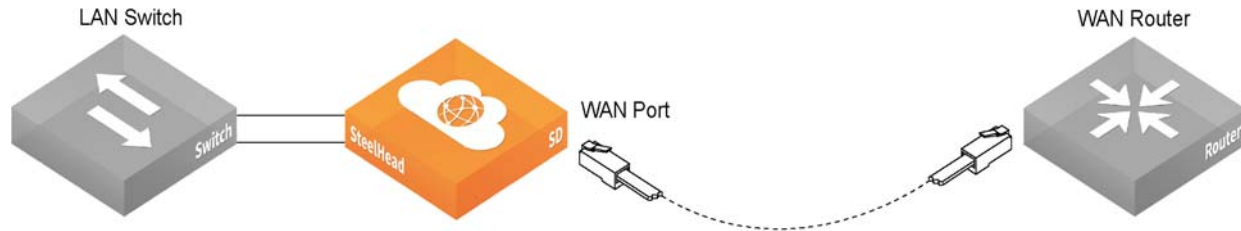
Figure 5-8. Connecting the WAN port to the WAN router
