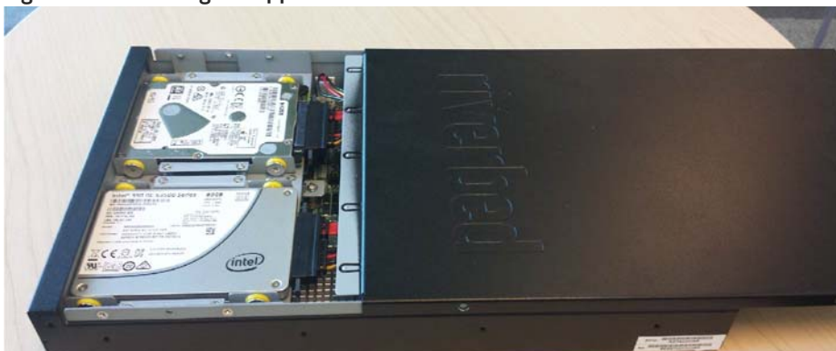
Figure 4-8. Installing the appliance cover
