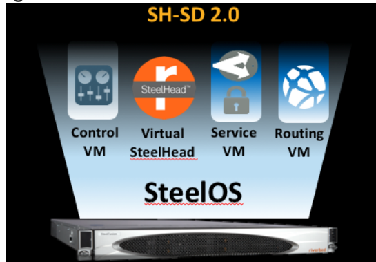
Figure 1-2. SteelHead SD software architecture
