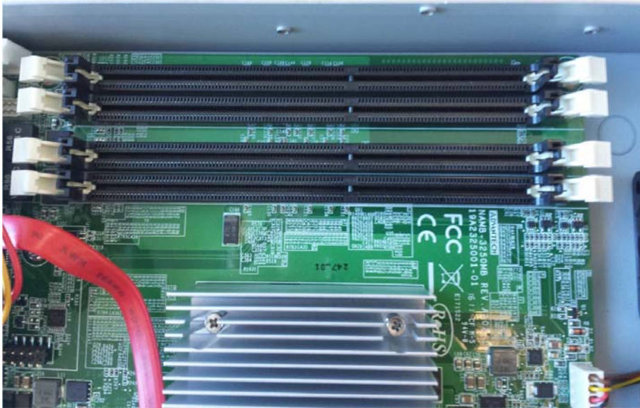
Figure 4-2. Locating the DIMM slots
