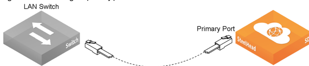
Figure 5-6. Connecting the primary port to the LAN switch
