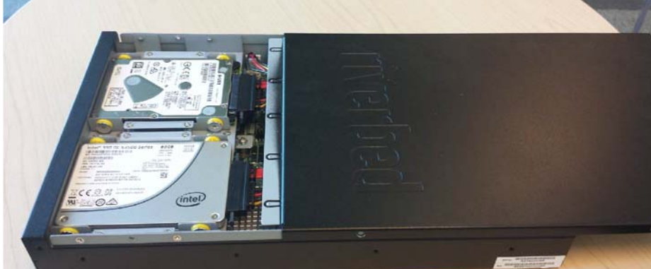
Figure 4-4. Installing the appliance cover
