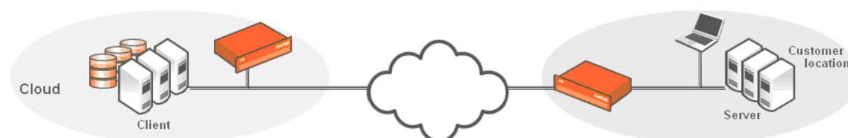
Figure 1-4. Clients in the Cloud Behind a SteelHead-c
