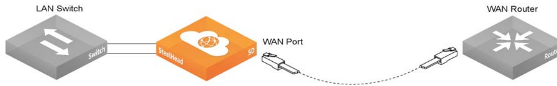
Figure 2-13. Connecting the WAN port to the WAN router
