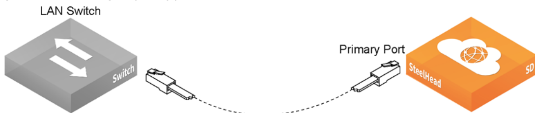
Figure 2-11. Connecting the primary port to the LAN switch
