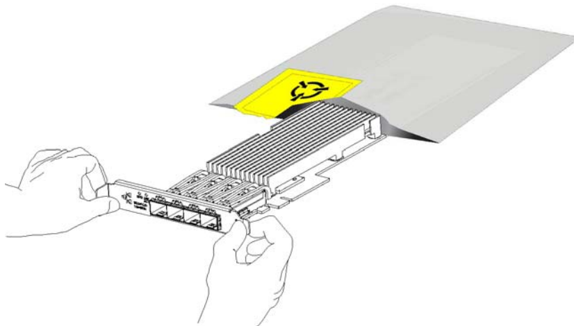
Figure 3-5. Removing the NIC from the ESD Bag
