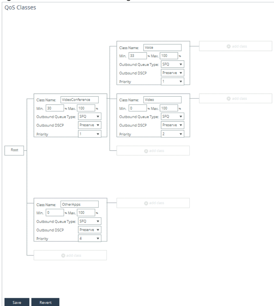
Figure 7-13. Finished QoS Class Configuration
