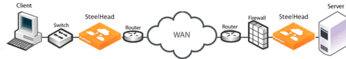
Figure 3-7. Firewalls and Transparent Addressing
